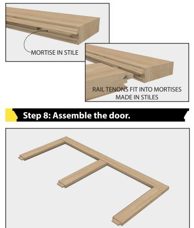
After routing the mortise-and-tenon joints, apply glue to all surface of the tenons and assemble the door. Insert the rails into one of the stiles as shown.
